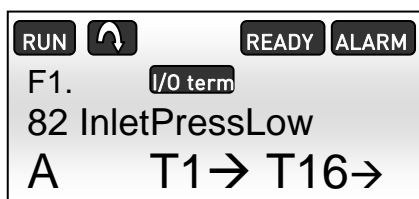
Figure 5.1-4, Low pressure alarm on the NXP panel
