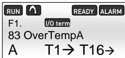
Figure 5.1-2, High temperature alarm on the NXP panel
